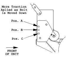
FIG. 16 DRIVE BELT TENSION ADJUSTMENT POSITIONS
